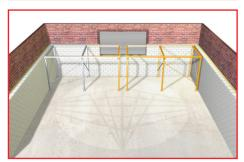
Stand two legs upright, align and insert each fin protrusion into each leg. Note that uprighted legs should never be left unsupported at any time. Legs are available in the following sizes:
