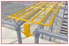
Use make-up panels to bridge gaps of up to 400mm between platforms and secure in place using Rhino Secure Ties, ensuring that the make-up panels are secured at the four corners, one tie at each corner. The makeup panels are designed to be used to bridge gaps between two or more platform systems for non-uniform plots.
